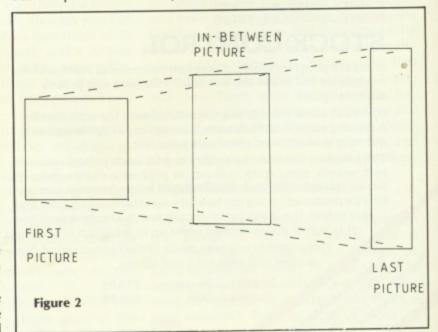
a FOR - NEXT loop controlled by the loop variable I, which takes values from 0 to F+1. If it only went from 1 to F, then only the F in-between frames would be drawn. When I is zero, the loop causes the first picture to be drawn... Setting 1 equal to zero in line 160, for example, reduces it to X2=XF(J). Similarly, when I is set to the value of F+1, the last picture is drawn, as a test corresponding to the one just described will show.
